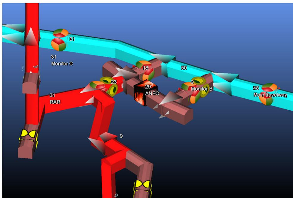
**FIG 2 - Magazine location and fire. Numbers are original airflows (m<sup>3</sup>/s) before fire.**
