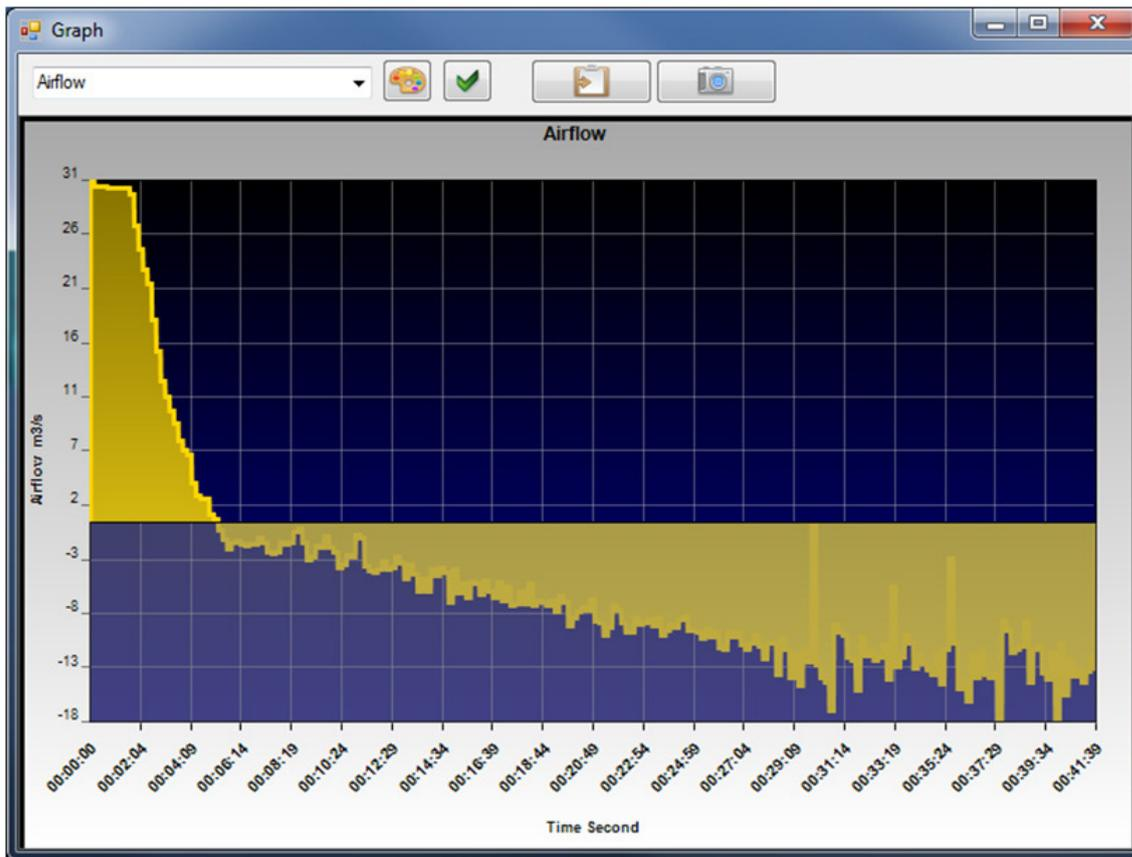
FIG 4 - Fuel bay output data at monitor A showing flow reversal.
